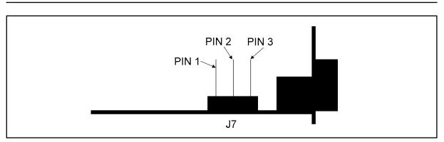
**Figure 24** XSlot Hot Sync card and jumper settings: Resistor ON: PIN 1 and PIN 2 connected, No resistor: PIN 2 and PIN 3 connected (default setting).
